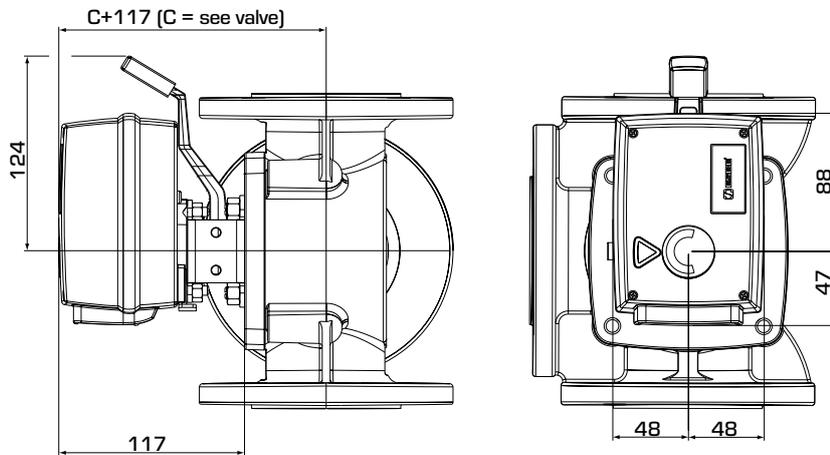
Installation dimensions for Actuator Series 90
