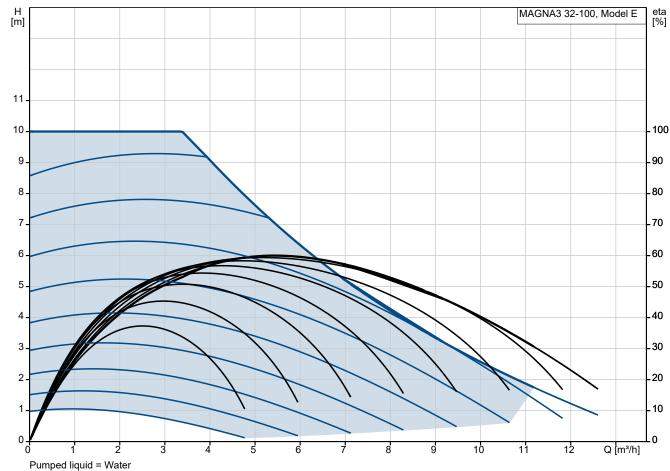
Eliquid temperature during operation = 60 °C Density = 983.2 kg/m<sup>3</sup>
