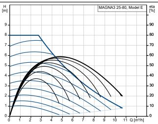
Pumped liquid = Water Liquid temperature during operation = 60 °C Density = 983.2 kg/m³
