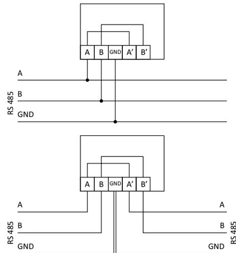
**Note:** A, B, A', B' and GND terminals are isolated from all other terminals.
