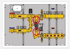
**NOTE.** For opening and closing operations use a screwdriver or a 5 mm Allen wrench.
