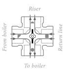
The flat-sided spindle top points towards the sleeve position.
