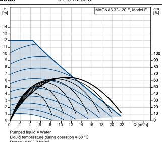
Liquid temperature during operation = 60 °C Density = 983.2 kg/m³
