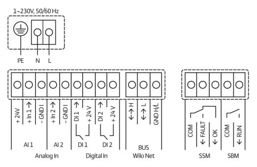
SSM: Collective fault signal (NC contact in accordance with VDI 3814, load capacity 1 A, 250 V ~)
