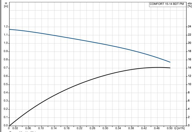
Pumped liquid = Water Liquid temperature during operation = 60 °C Density = 983.2 kg/m³
